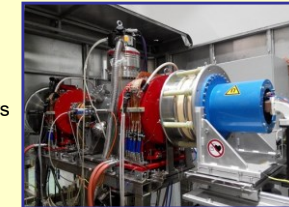
High-intensity neutron generator producing about 10^{12} neutron/s (~ 2,8 W fusion power) Consumed power to operate: ~40 kW
